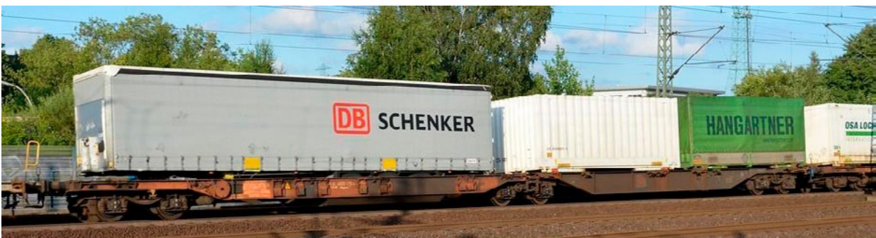
Example of a train carrying semi-trailers and containers with Sdggmrss T3000e wagons.
