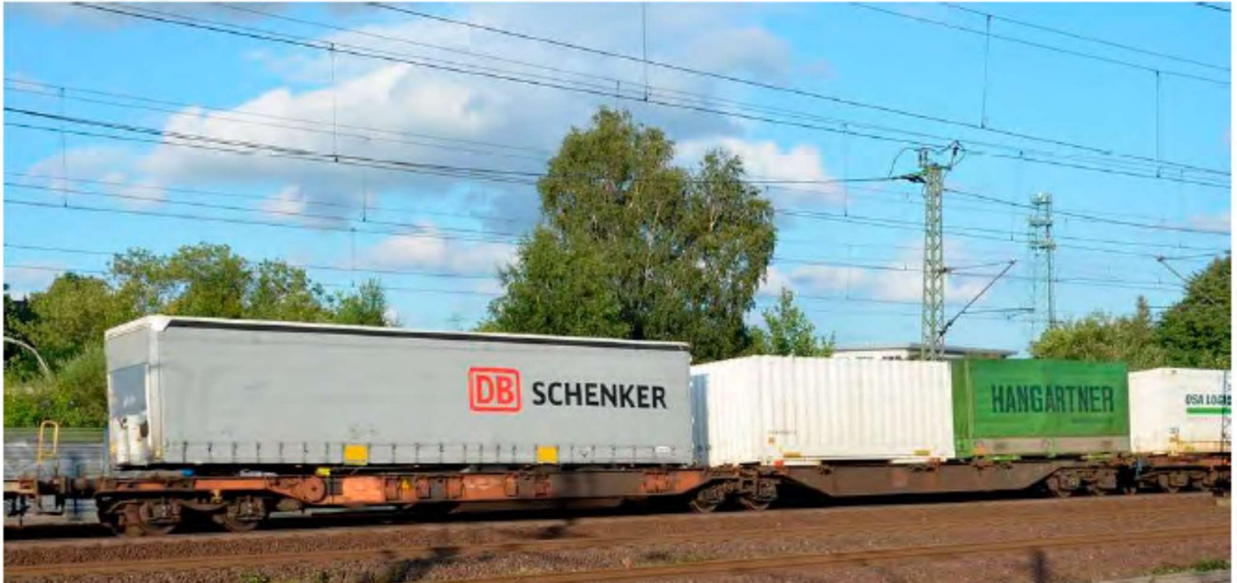
Sdggmrss, T3000e wagon loaded with a semitrailer and two 20' containers
