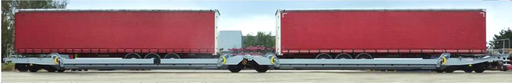
Wagon designed to carry standard semi-trailers.
