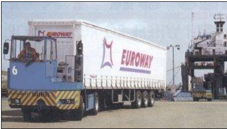
Fig. 6.34: Tugmaster or Terminal Tow Tractor used for handling of semitrailers in ports and for loading / unloading of RoRo-ferrries (Photo: Port Logistics Ltd.)
