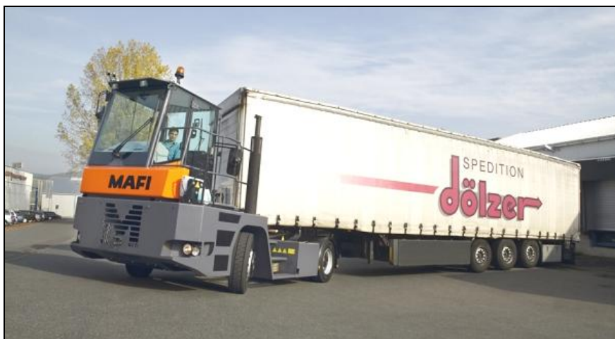
Fig. 6.35: Tugmaster or Terminal Tow Tractor used for handling of semitrailers in terminals and ports (Photo: MAFI GmbH)
