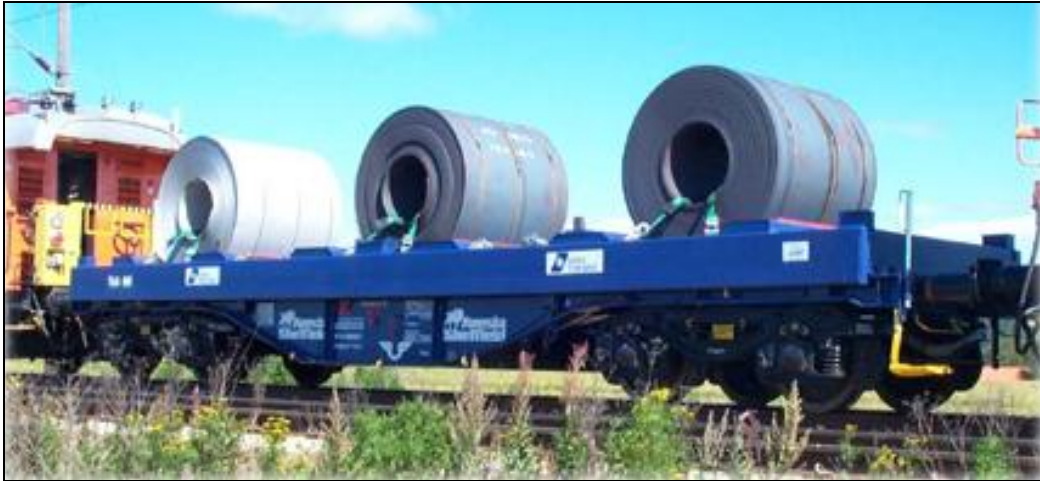
Fig. 6.22: Swedish class Sgmmns-w wagon with a detachable cassette loaded with coils (Photo: Kockums Industrier)
