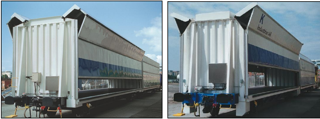
Fig. 5.20 + 5.21: Hiqrrs-vw 011 (left) and its European version Hiqrrs-vw 041 (right). The photos reveal the almost rectangular cross-section of the Swedish version, creating the condition for an efficient utilization of the loading space, while the European version is characterized by “cutted” upper corners in order to adhere to the G2-gauge (Source: K-Industrier)
