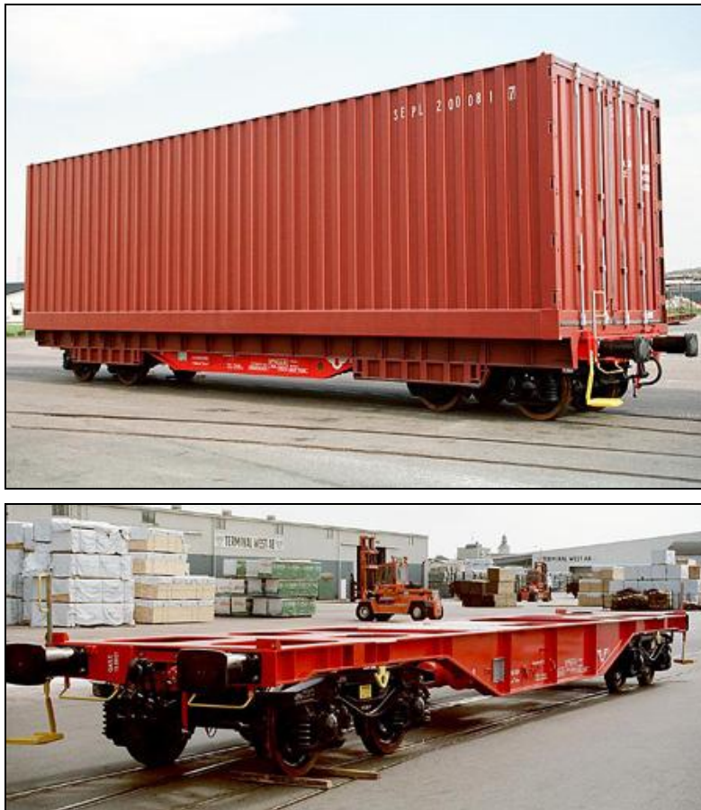
Fig. 5.23 + 5.24: Wagon of class Sgmns-w 982 loaded with a SECU loading unit (above) and empty (below). (Source: Stora Enso, K-Industrier)
