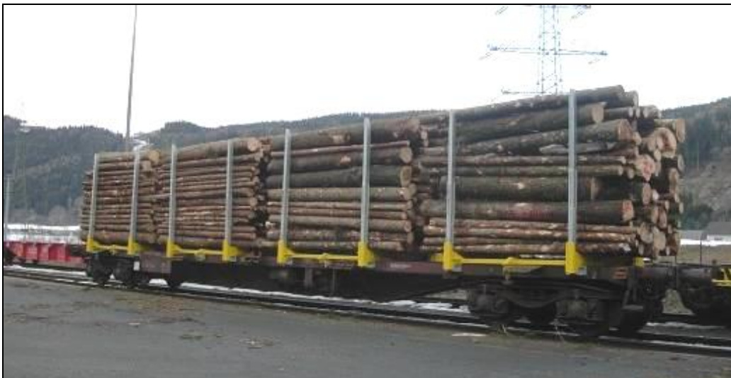
Fig. 6.1 + 6.2: Standard container wagons in Sweden (above) and Austria (below) equipped with semi-permanently fixed stanchions allowing the wagons to be used in timber traffic.
