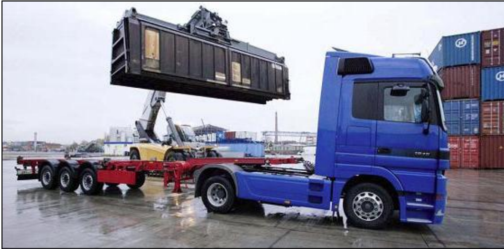
Fig. 6.5: Detachable superstructure of a railway wagon, which can be handled by standard terminal handling equipment.
