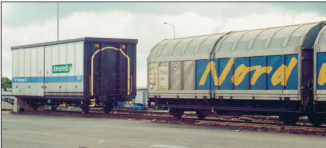
Fig. 5.30: Prototype covered wagon utilizing the same loading gauge as the SECU-trains. Note the yellow line indicating the cross-section of a standard freight wagon (Source: TfK)
