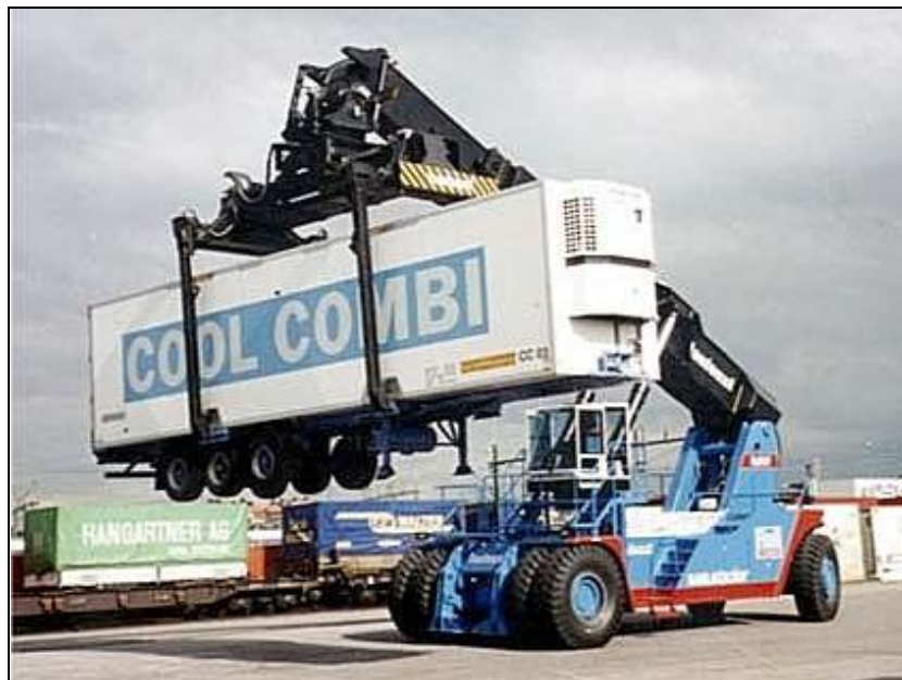
Fig. 6.33: Loading of a semitrailer onto a rail wagon by reachstacker with help of spreaders. The trailer needs to be equipped with side gripping pockets. Only
