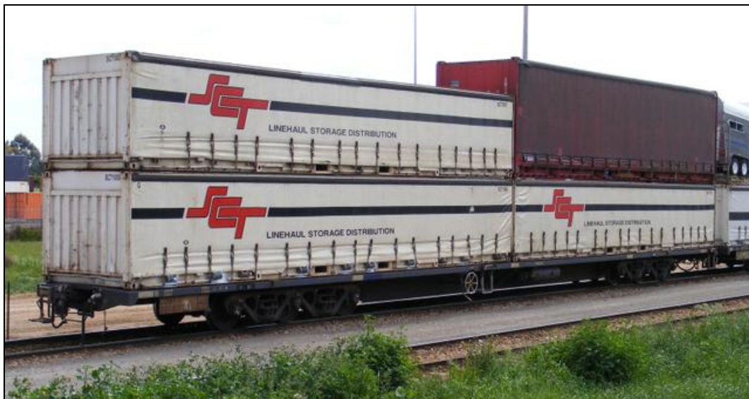
Fig. 5.12: Australian 80'-class CQMY wagon loaded with four 40'-loading units, equivalent to 8 TEU. (Source: www.railpage.com.au )
