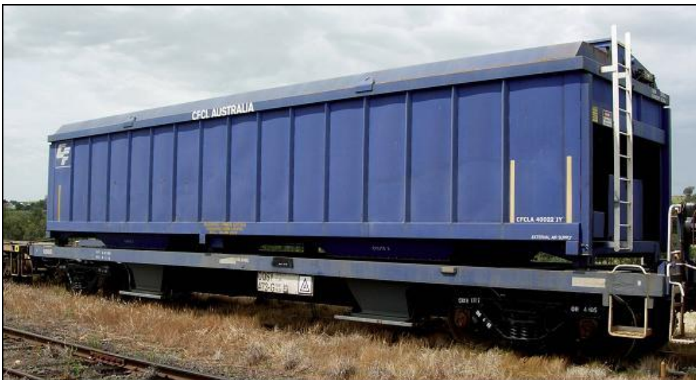
Fig. 6.3 + 6.4: Different type of non-ISO loading units, which can be carried on container wagons.
