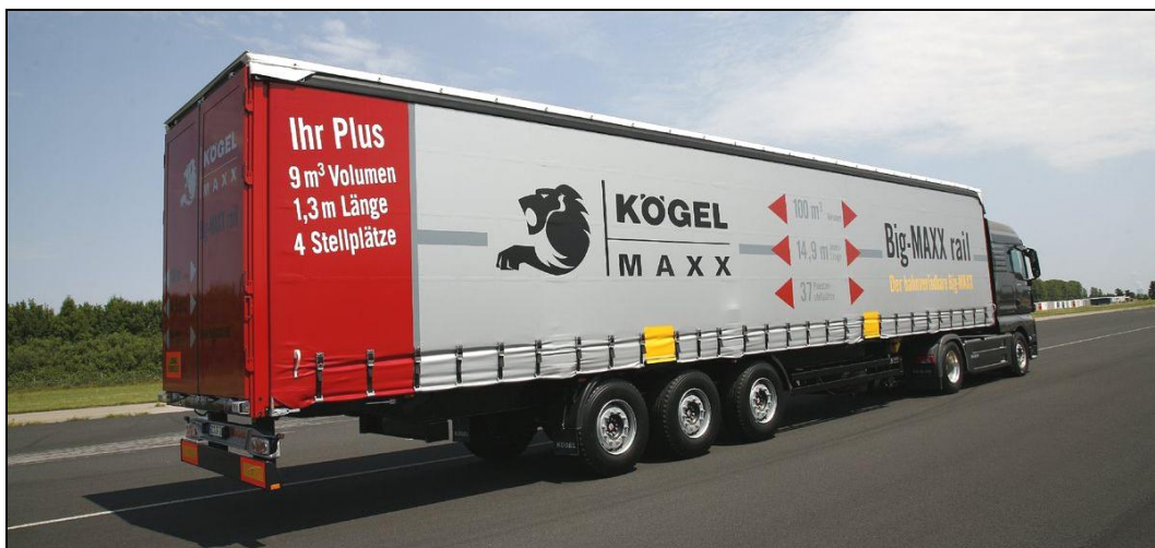
Fig. 6.28 + 6.29: Standard 13,68 m semitrailer (above) and 14,92 m long prototype semitrailer from KÖGEL. The trailer length defines the length of the TOFW-wagon (Photo: Valerius, Kögel).
