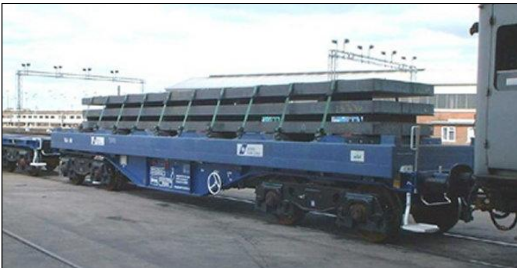
Fig. 6.23: British class BVA-wagon – almost identical to the Swedish Sgmmns-w wagon – with the same detachable cassette as in the previous figure, but here loaded with steel slabs (Photo: Kockums Industrier)
