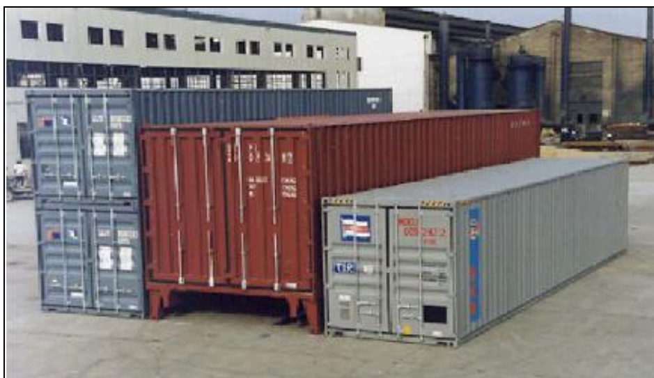
Fig. 5.28: SECU loading unit in comparison with standard ISO-containers (Source: Port of Göteborg)
